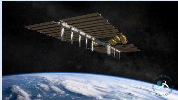
*Figure 3. LEO propellant depots produce propellant from water delivered from Earth and refuel Space tugs.*
